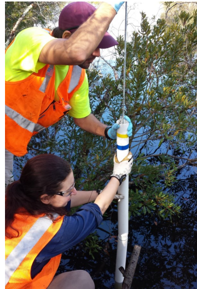
Sediment Bed Passive Flux Meter (SBPFM): CH2M HILL conducted a study in Wallace Creek to evaluate the effectiveness of a SBPFM to test and validate whether the technology can be successful in the field to measure the exchange water between the creek and subsurface.
