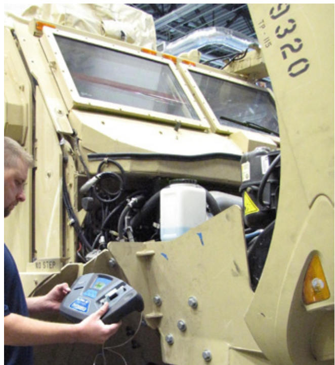
Refrigerant electronic testers are used on tactical vehicles to analyze refrigerant purity and identify equipment that has been contaminated with counterfeit refrigerants.
