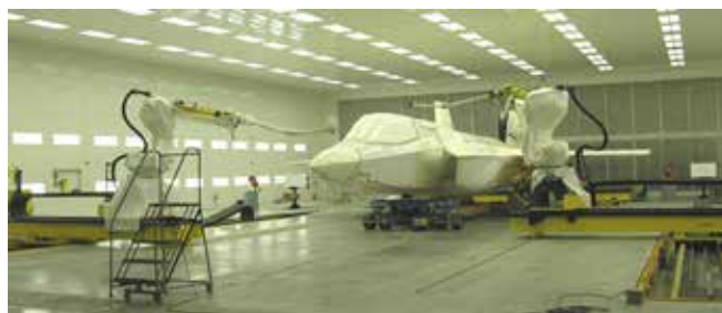
Pictured here is a robotic painting work cell. A new lightweight coating system eliminates one layer of paint from the traditional system resulting in an overall aircraft weight reduction and over 50-percent reduction in the paint/paint-removal waste stream.
