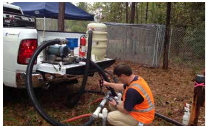
A remediation technology study is being conducted (pictured here) to evaluate potential groundwater treatment alternatives for selection of a final remedy. The study resulted in a reduction of concentrations to below detection limits within one month of start-up.
