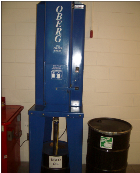
Fuel and oil filter crushers are part of recycling efforts at FMS 2. The crushers allow the P2 Team to reclaim petroleum products for recycling and allow used filters to be recycled as scrap metal rather than disposed of as hazardous waste. Antifreeze is also recycled with help from an outside recycling vendor.
