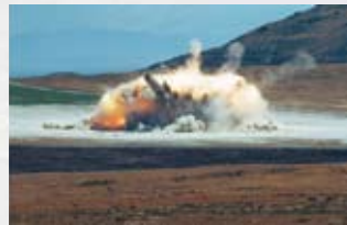
EQT and range staff successfully demilitarized the first Trident first-stage rocket motor (81K lbs net explosive weight).
