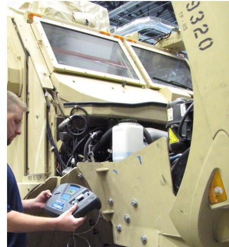
Refrigerant electronic testers are used on tactical vehicles to analyze refrigerant purity and identify equipment that has been contaminated with counterfeit refrigerants.
