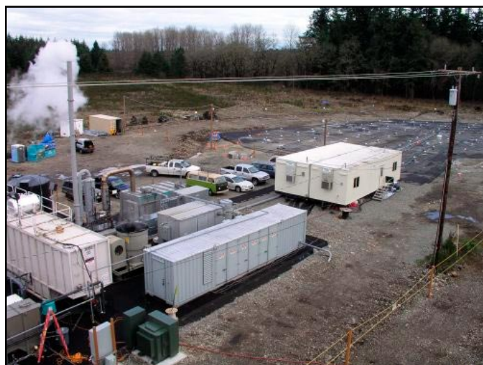
Electrical resistance heating, an in-situ technology, in use at the Logistics Center NPL site.
