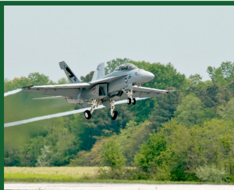
Figure 1: Supersonic Flight Test of the F/A-18 Super Hornet Strike Fighter Jet powered by a 50/50 biofuel blend.
