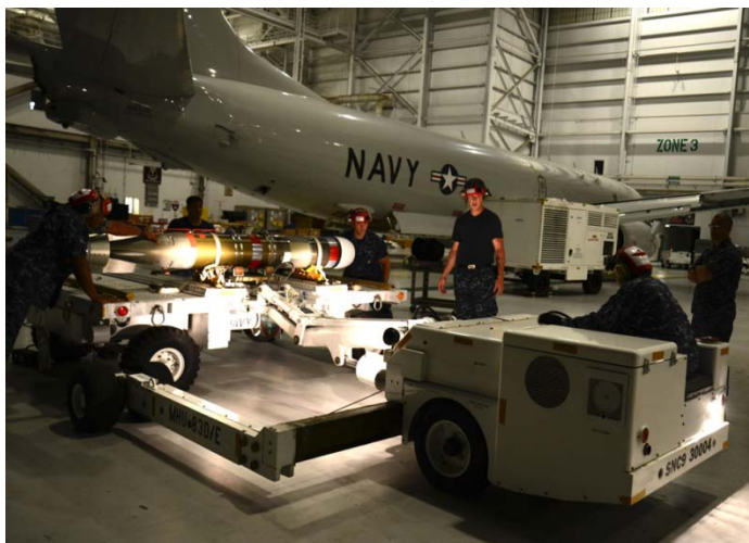
Figure 2: Patrol Squadron (VP) 16, prepare to load a MK-54 torpedo onto a P-8A Poseidon aircraft in Jacksonville, Fla.
