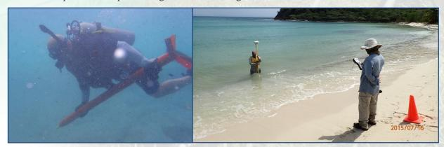
Figure 9: Diver placing a munitions surrogate on the ocean floor (left photo). Survey team measuring monthly changes in beach conditions (right photo). The combined information from this first-of-its-kind beach dynamics investigation will be crucial in predicting changes in beach conditions and the munitions that reside on, under, and adjacent to them. This information will then be used to plan the most cost-effective remedial actions.
