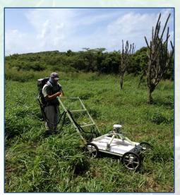
Figure 7: Finding and discriminating subsurface anomalies with TEMTADS. Successful testing in Vieques has helped support the use of this technology at other bases, and the TEMTADS is planned for fullscale implementation in Vieques in 2016.
