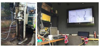
In general, high EC readings indicate clayey lithology and high HPT pressures indicate low permeability lithology. At each borehole where HPT/EC logging was conducted, three to four dissipation tests were conducted to approximate the absolute hydrostatic pressure. The dissipation test data were used in
