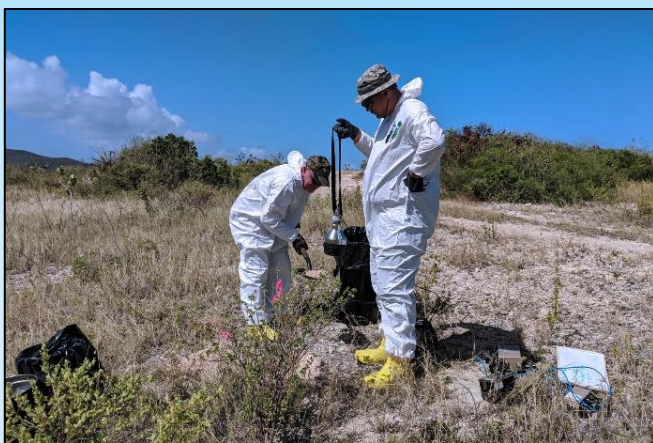
Figure 7. Team comprising radiological and UXO specialists locate and remove depleted uranium projectiles and collect soil samples.
