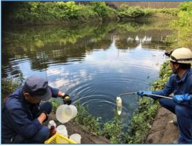
**Stormwater Sampling** As part of a JEGS' annual requirement, Naito Environmental contractors are sampling to make sure the stormwater on YAB does not contain any harmful chemicals that could drain into the Tama River.
