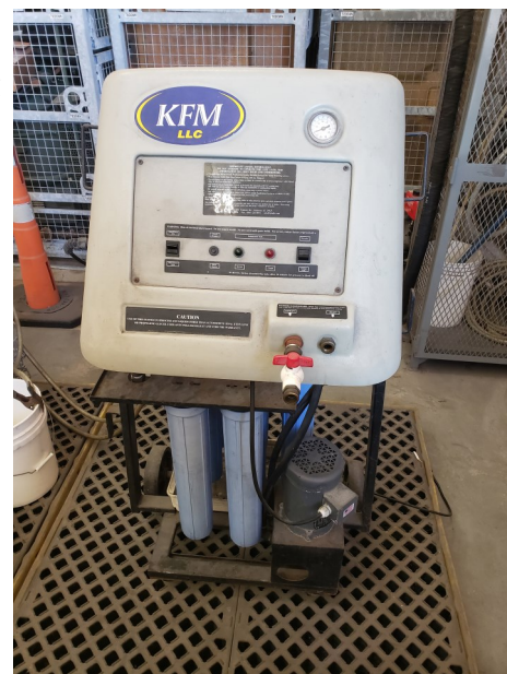
KFM, LLC coolant purification system used to recycle used antifreeze at MCSF-BI. Used antifreeze is collected by shop personnel and transferred into a used antifreeze tank at Building 350. Once a sufficient volume of has been collected, it is processed through the coolant purification system and transferred into a purified antifreeze tank for dispensing to shops.
