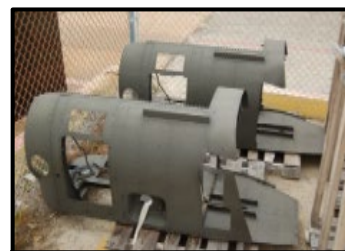
Zirconium Pretreatment Replaces Chromated Conversion Coatings (immersion and spray-on)
