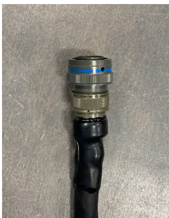
The U.S. Army Combat Capabilities and Development Command Safer Alternatives for Readiness program is conducting research and development to replace Cr6+ containing electrical connectors with a greener, safer alternative. The left photo is an example of a current system Cadmium/Cr6+ connector. The right photo is a connector which uses Black Zinc Nickel as a possible alternative coating.
