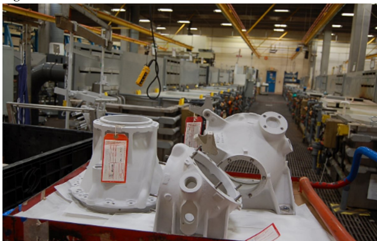
Three magnesium housings coated with Tagnite. Tagnite is an alternative pretreatment to the legacy Cr6+ conversion coatings. It is not only a safer alternative but it also provides superior corrosion protection over the legacy process.
