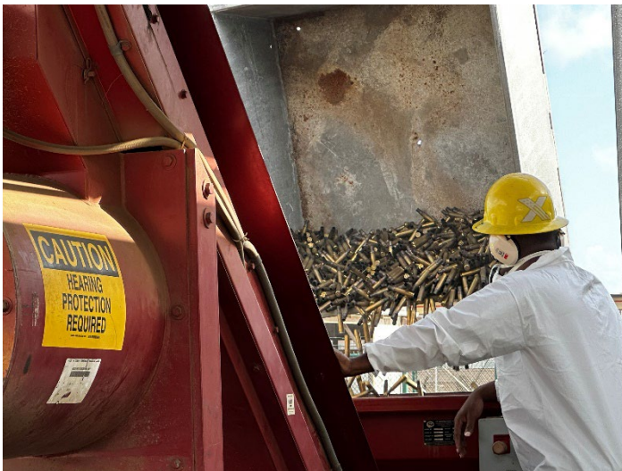
Expended small arms cartridge casings (ESACC) is emptied from a storage bin into a brass deformer while a QRP employee monitors the process.
