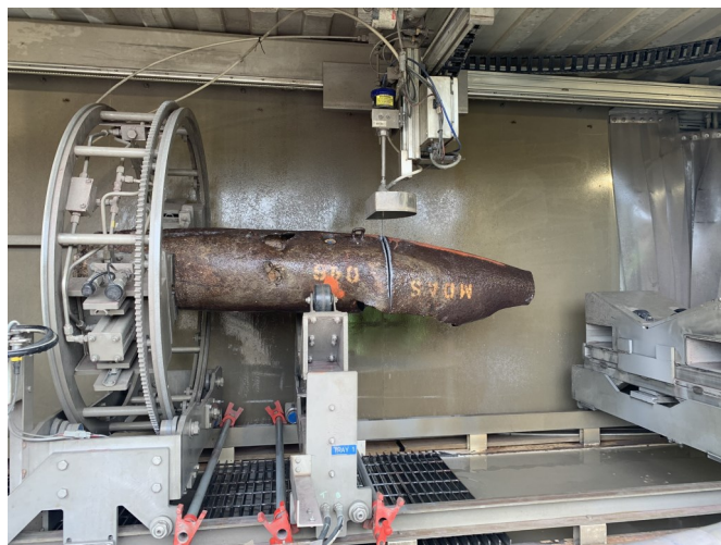
Water jet cutting system dismantling an inert practice bomb recovered during the munitions cleanup in Vieques. Processing inert munitions in this manner is a cost-effective way to enable the metal casings to be recycled for beneficial reuse.
