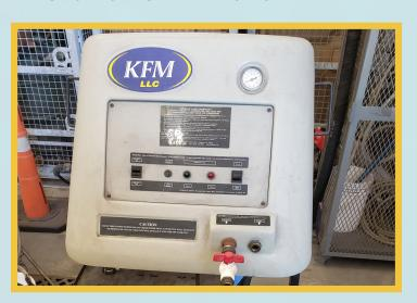
The KFM, LLC coolant purification system is used to recycle used antifreeze at Marine Corps Support Facility Blount Island. Shop personnel collect used antifreeze and transfer it into a tank. Once a sufficient volume is collected, it is processed through the system and transferred into a purified antifreeze tank for dispensing to shops.
