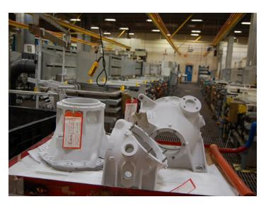
Three magnesium housings coated with Tagnite. Tagnite is an alternative pretreatment to the legacy Cr6+ conversion coatings. It is not only a safer alternative but it also provides superior corrosion protection over the legacy process.
