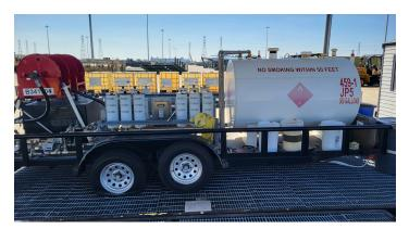
The Fuel Filtration Unit (FFU) at MCSF-BI, with several off-spec JP-5 totes visible in the background. The FFU can process most off-spec fuel generated at MCSF-BI. However, contaminated fuel cannot be processed through FFU, and is turned in to the Mayport Base Operating Support contractor for management as waste.
