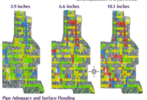
Stoplight map of pipe adequacy and surface flooding in Minneapolis.
