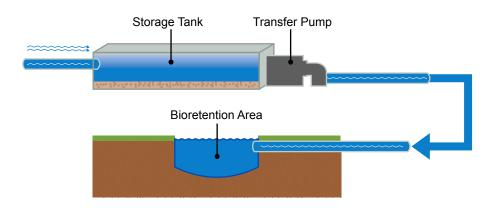
System diagram of the prototype installed at the Perry Center: stormwater flows into a storage tank where debris are settled. A pump transfers water based on the level to a downstream bioretention cell.
