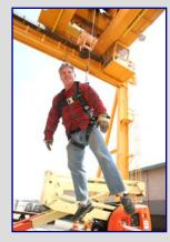
Two eight-inch I beams, six trolleys and trolley stops attached to the underbelly of an Ederer 200-ton overhand bridge after retrofit with *self-retractable lifeline* fall protection system.
