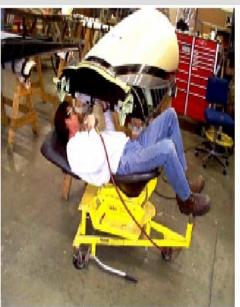
The tilting seat of the industrial positioner provides proper body support
