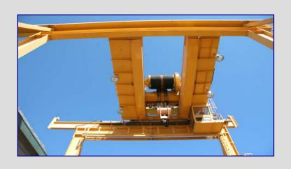
200-ton Ederer overhead bridge crane before it was outfitted with self-retractable lifeline fall protection devices. Riggers had to climb out onto the component to attach rigging device to the crane hook.
