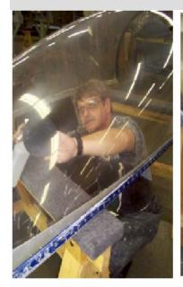
Mechanic having difficulty working on underside of canopy before ergonomic improvements
