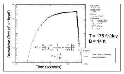
Figure 2a: Vacuum versus Time Data and Transient Model Analysis using AQTESOLV® Software
