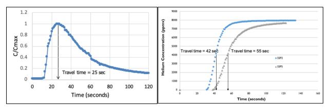
Figure 3: Tracer Test Plots for Inter-Well Test (3a, left) and Flood Test (3b, right)
