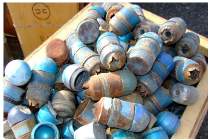
Training grenades have a small explosive charge that upon functioning causes a "flowered" opening on the bottom. Training grenades are similar in appearance to grenades with either a solid aluminum slug or a high explosive-fill.
