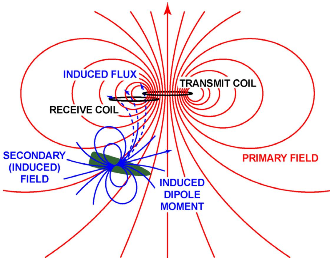
Figure D-10. Electromagnetic Induction (EMI)
