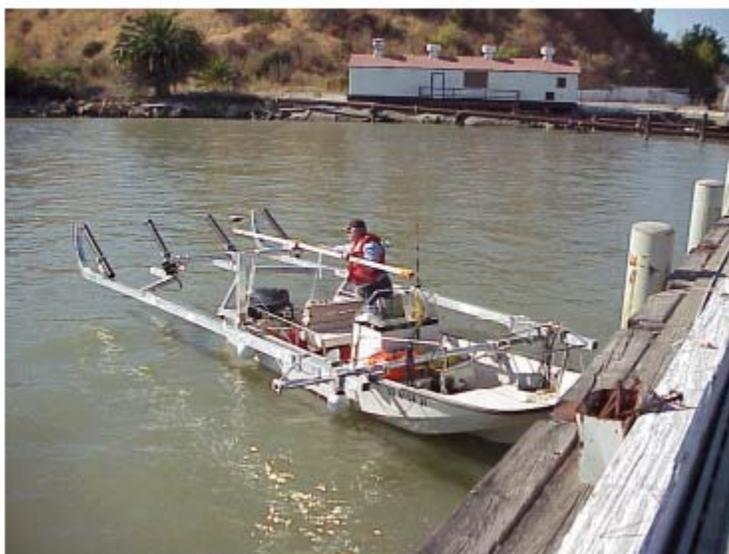
Photo 5. Alpha Geoscience/SONTEC mounted AGS-2 Magnetometer.
