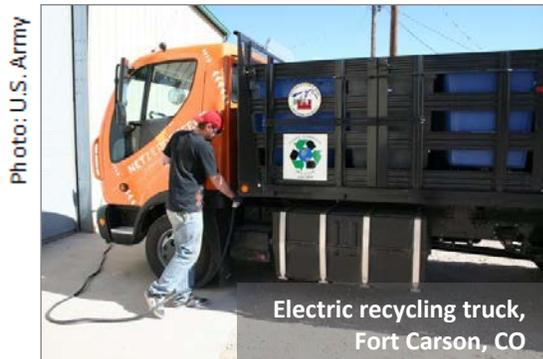
The Army will continue its vehicle-to-grid technology efforts, including a pilot project at Fort Hood (TX) in FY 2016, deploying charging stations to support the installation’s hybrid-electric trucks and EVs. The system can provide demand response, peak shaving, and ancillary services in addition to limited emergency backup power to critical functions. As part of a pilot program with GSA and CEQ, the Army committed to
