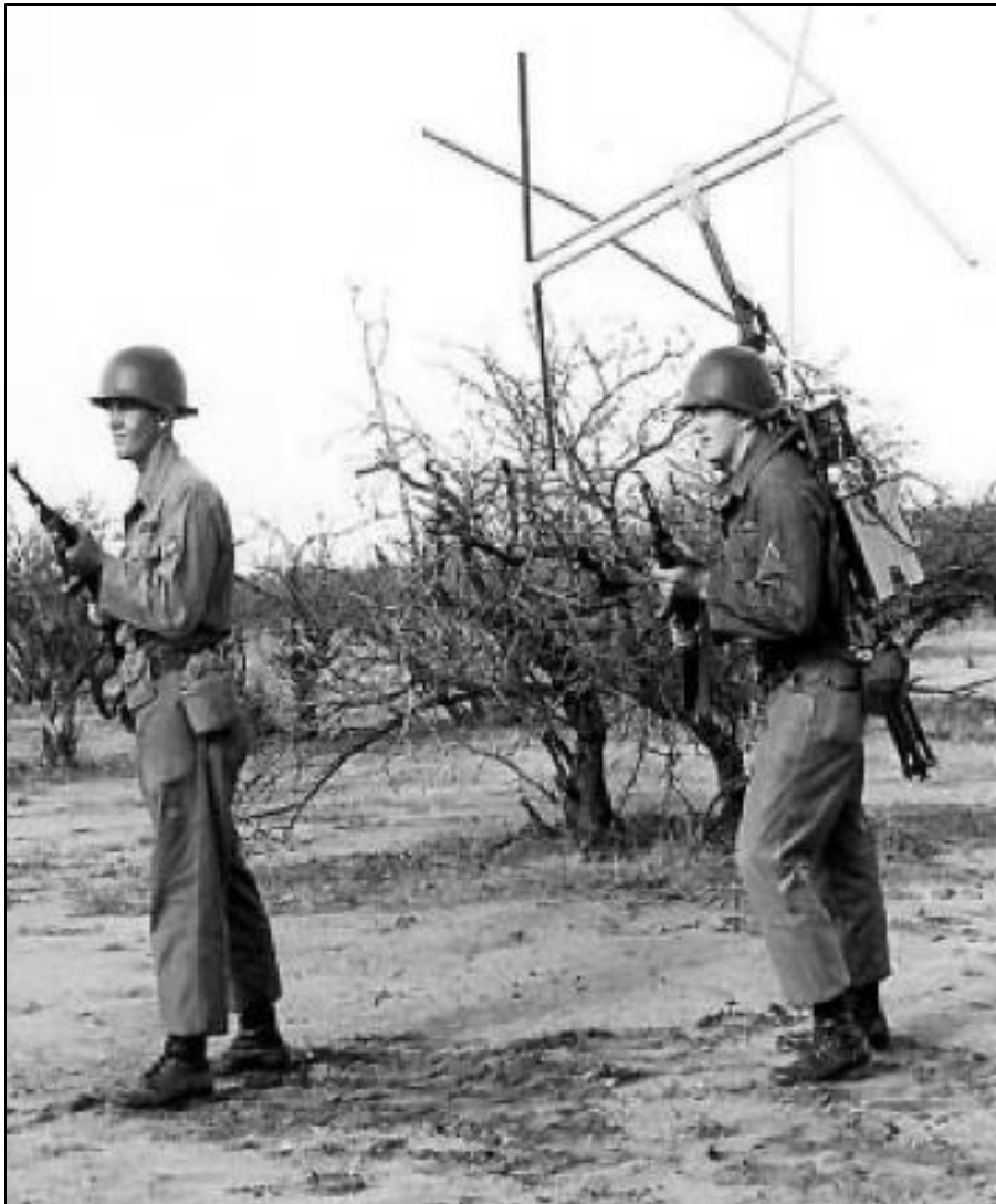
Figure 79. Soldiers wearing the experimental model of the Manpack Jammer EP/EDL-39 at Fort Huachuca, Arizona, 1960.
