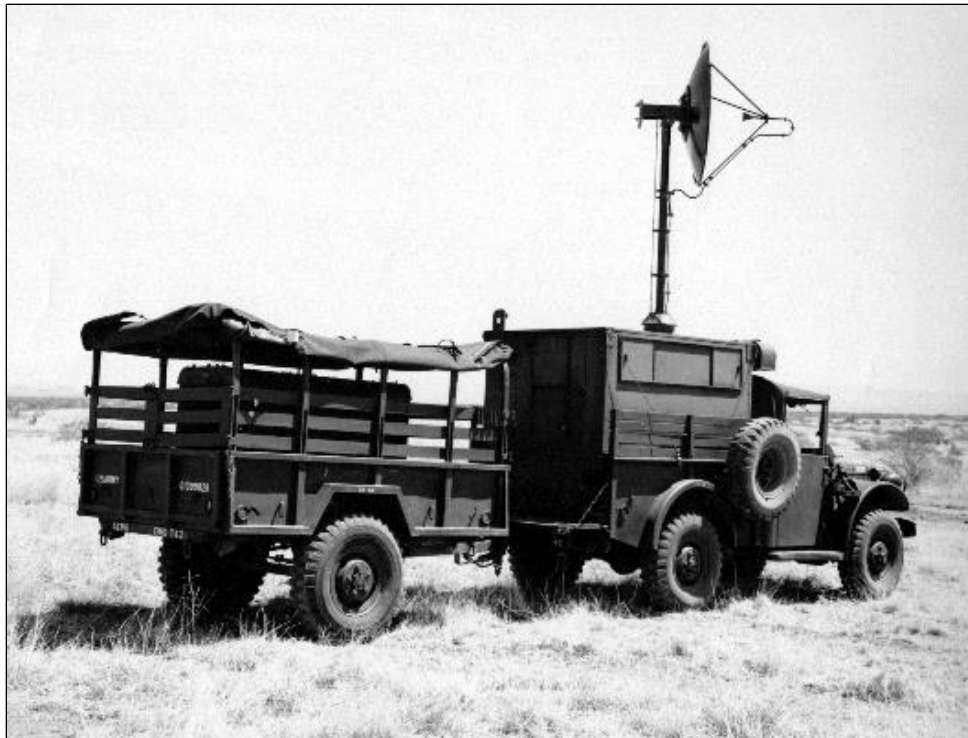
Figure 61. The EPG Electronic Warfare Department evaluated the first experimental model of K-band jammer, shown, 1959.
