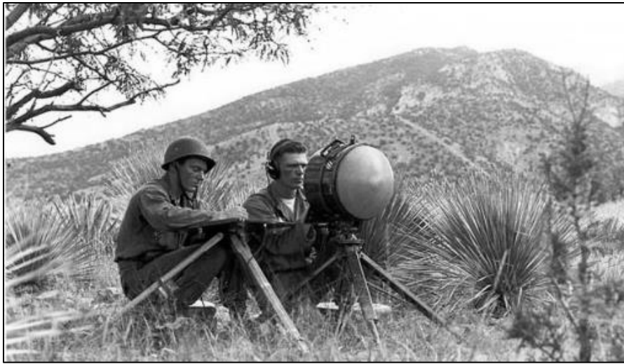
Figure 75. The compact, all-weather radar “eye” (AN/PPS-4 Radar Set), which detected motion in variable conditions, was field tested at Fort Huachuca (AN/PPS-4 Radar Set), 1956.
