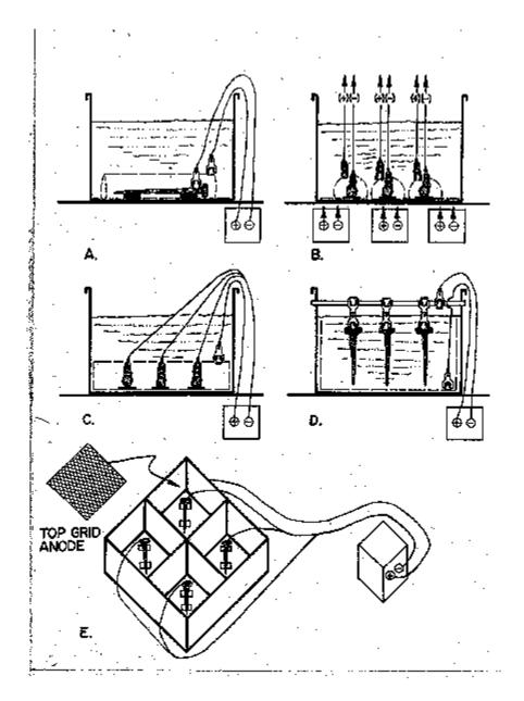
Figure 5. Electrolytic Reduction Setups.
