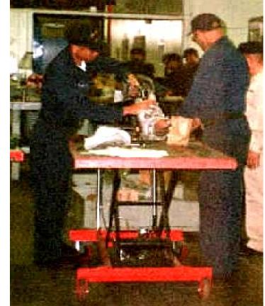
Portable scissors lift table is used a: work bench which eliminates awkward postures and excessive lifting
