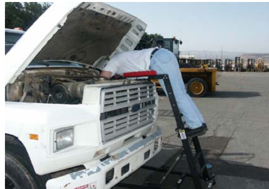
Intervention: Topside Creeper
