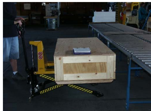
Intervention: Scissor Lift Pallet Jack
