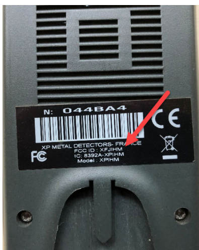
Figure 15: A label with the FCC Id on an electronic product
