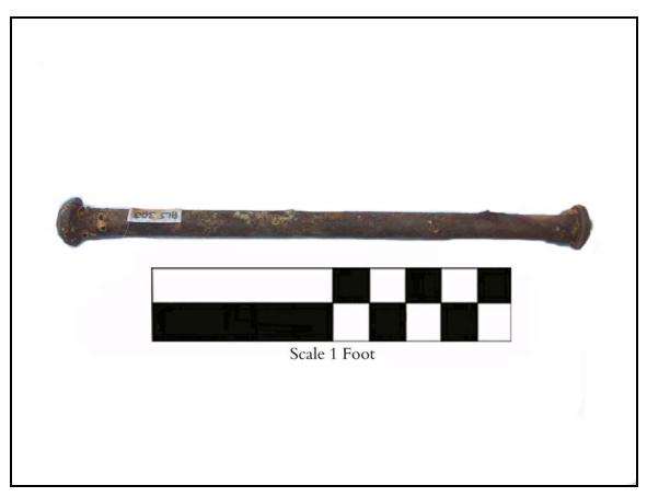
Figure 48. ALS-303 Fastener with rove.
