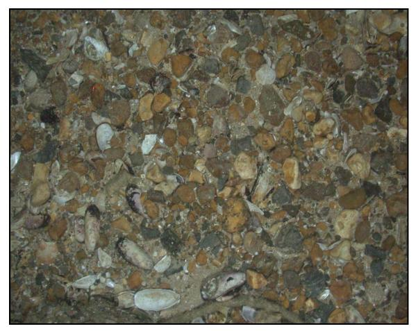
Figure 6. Sample of bottom surface sediment at the CSS Alabama wreck site.
