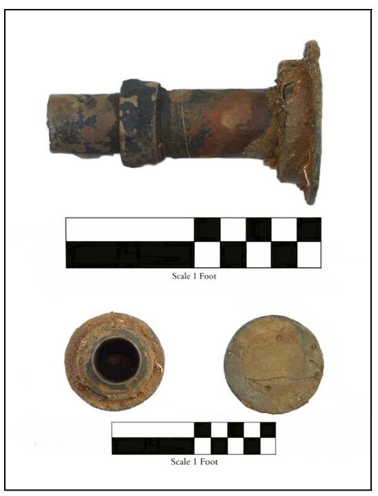
Figure 46. ALS-300 Fill pipe, deck flange and cap.
