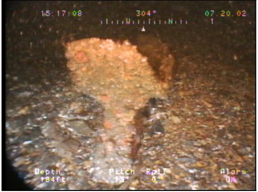
**Figure 25.** Fluke of the port Trotman anchor.
