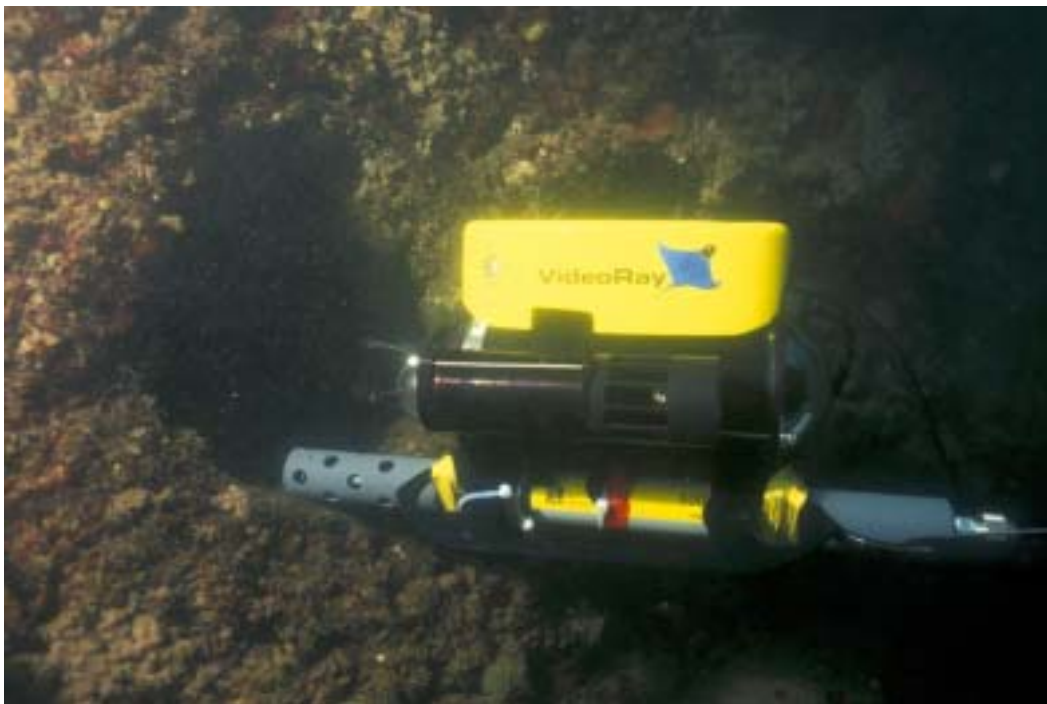
Figure 12. VideoRay ROV equipped with YSI sonde entering porthole on Arizona 's second deck.
