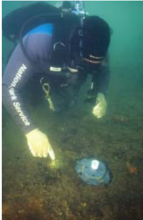
Figure 14. NPS archeologist installing new GPS monitoring point (right) adjacent to the old point (left).
