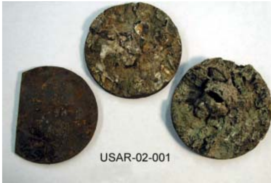
Figure 2. Hull “coupon” with interior and exterior concretion. Note the “chord” cut from the steel sample on left.
