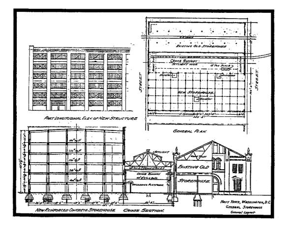
Figure 2. Plate showing cross section and partial elevation of general storehouse constructed at Washington Navy Yard, D.C. (U.S. Navy Department, Bureau of Yards and Docks, *Public Works of the Navy, Bulletin 23*, June 1916:22) Drawing depicts contrast between storehouse constructed before 1916 and storehouse constructed in 1916.
