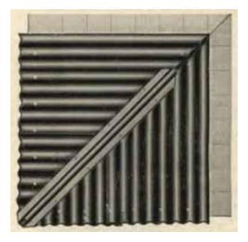
Illustration 15: A roof plan view of corrugated metal roofing on a hipped roof with a ridge cap (Milwaukee Corrugating Co. 1920:147).
