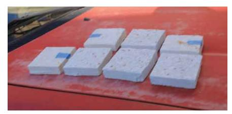
Illustration 65: The concrete mock-ups for the patching to Building 3. Each sample varies slightly in color and/or aggregate type (Photographer: Samantha Driscoll 2015).
