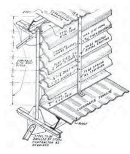
Illustration 37: Asbestos-cement panels were also made into louvers for industrial applications requiring extra ventilation (Johns-Manville 1944:22).
