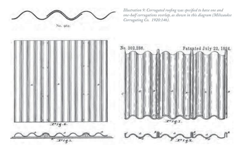
Illustrations 10 and 11: Comparison of the overlapping corrugation connection method (left) and the "V-crimp" connection method (right). The overlapping corrugation method remains the preferred connection method (U.S. Patents 1884:302286 A).
