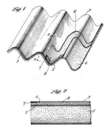
Illustration 29: An example of a reinforced asbestos-cement panel, with a layer of textile between two asbestos-cement boards (U.S. Patents 1943:2335208 A).
