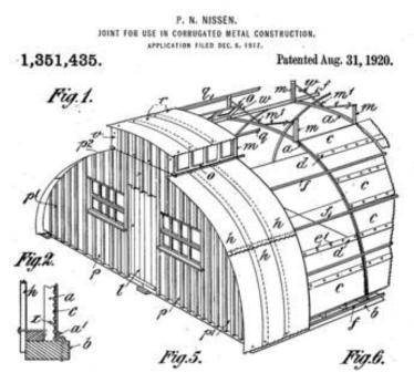
Illustration 19: Captain Peter Nissen first developed the Nissen Hut in 1916, fabricated with corrugated iron. The U.S. patent was filed in 1917 (U.S. Patents 1920:1351435 A).
