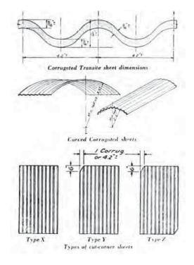
Illustration 23: Details of corrugated asbestos-cement panels (Johns-Manville 1944:9).
