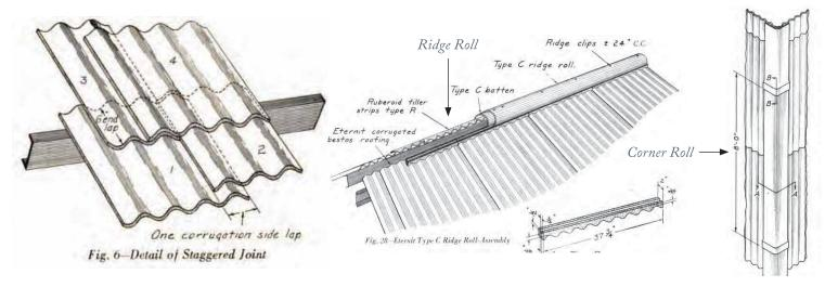
Illustration 32: The joints of corrugated asbestoscement panels were staggered to prevent leaks (Ruberoid Co. 1930:9)
