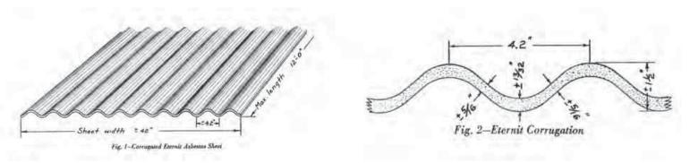
Illustrations 25 and 26: Corrugated asbestos-cement panels could be used for roofing or siding and had the strength to accommodate longer spans (Ruberoid Co. 1930:7).
