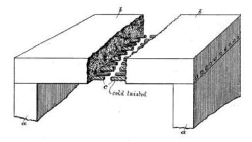
Illustration 3: Ernest L. Ransome's patented design for cold-twisted iron reinforcement in concrete (U.S. Patents 1894:516113 A).
