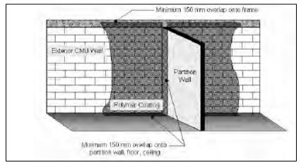
Figure 34. Polymer coating overlapping structural components (ETL 02-4).
