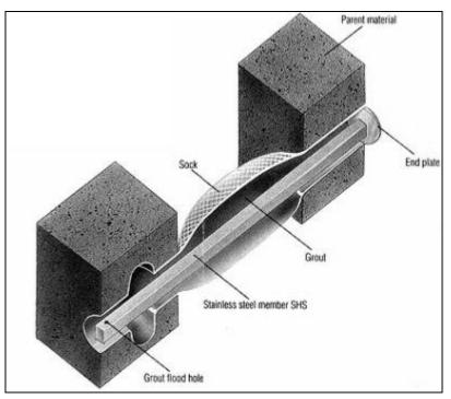
Figure 31. Retrofitted Reinforcement by means of coring (Sanicki 1998).
