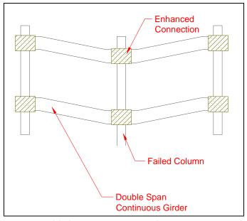
Figure 21. Conceptual diagram of catenary action.
