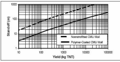
Figure 33. Comparison of standoff required for CMU walls with and without sprayed polymer coating (ETL 02-4).
