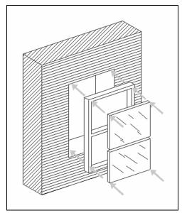
Figure 40. Blast load path through a window system.
