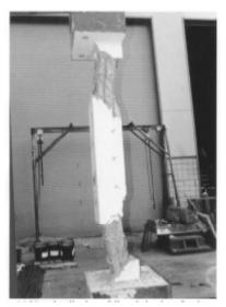
Figure 15. Buckling of an unwrapped reinforced concrete column (Crawford, Malvar, and Morrill 2001).
