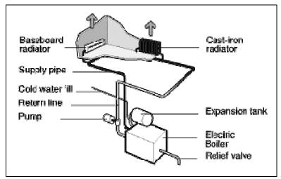
Figure 49. Radiator loop system (Hayden 1996).
