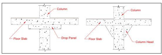
Figure 23. Details of drop panel and column head connection enhancements.
