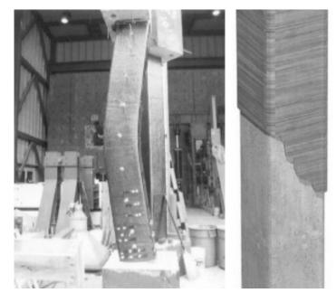
Figure 18. Column ductile performance enhanced by CFRP hoop wrap (left); wrapping detail (right) (Crawford, Malvar, and Morrill 2001).
