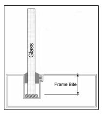
Figure 42. Diagram showing frame bite.
