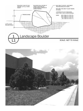
Figure 5. Boulders can be used to thwart vehicle access if they are part of the historic context (USAF 2006).
