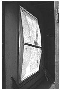
Figure 45. Flexible frame blast-resistant window with collapse mechanism at mid-window (Oldcastle-Arpal, not dated).
