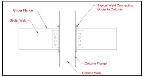
Figure 13. Conventional welded structural steel frame beam/column connection.
