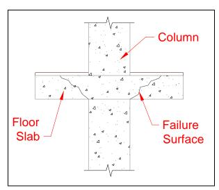
Figure 22. Conceptual diagram of punching shear.
