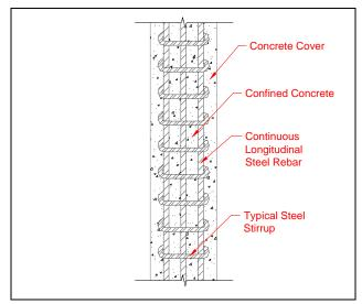
Figure 14. Components of a reinforced concrete column.
