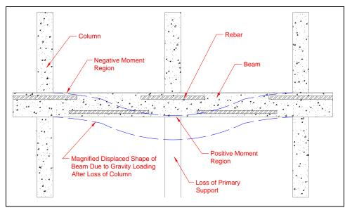
Figure 27. Reinforced concrete beam response to column loss.
