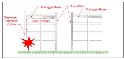
Figure 25. Outrigger beam and belt load-carrying system.
