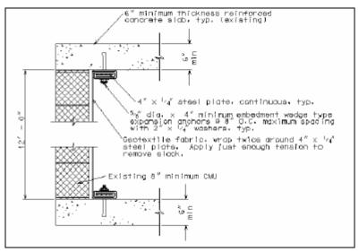
Figure 36. Cross section of geotextile fabric installation (ETL-1110-3-494).
