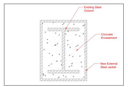
Figure 16. Steel column with concrete-filled steel jacket.
