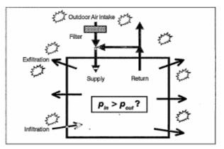
Figure 53. Pressurization/filtration protection (Persily 2004).
