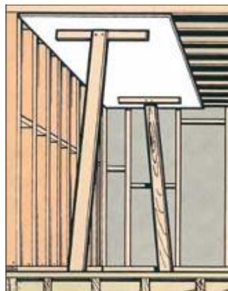
Diagram on how to properly use T Braces to support loose plaster. Source: http://static.howstuffworks.com
