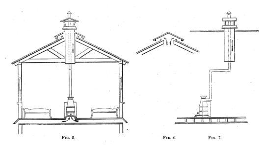
Figure 114. Drawings of ventilation schemes for the Circular #10 hospitals (NARA Washington, DC, RG 112, Entry 63, Box 3).
