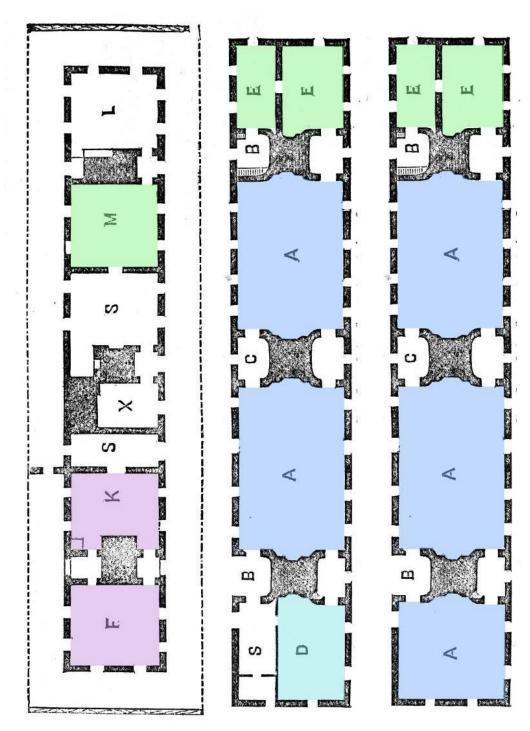
Figure 38. Jefferson Barracks, Missouri hospital floor plan [left basement, middle  $1^{st}$  floor, right  $2^{nd}$  floor] 1875 (Circular #8).
