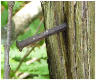
Machine-cut nail embedded in fence post (ERDC-CERL 2013).
