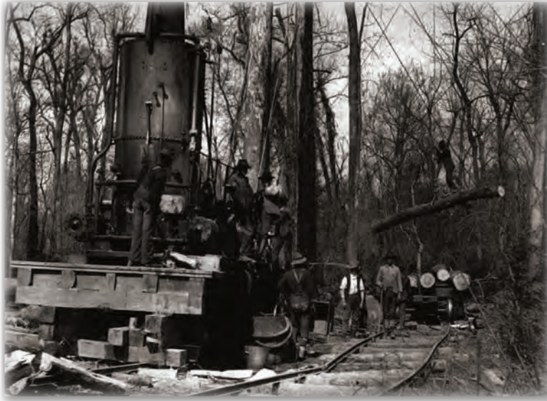
Steam Powered Skidder. In this photograph, the equipment is being used to load logs onto a rail car. South Carolina, 1904 (U.S. Forest Service).
