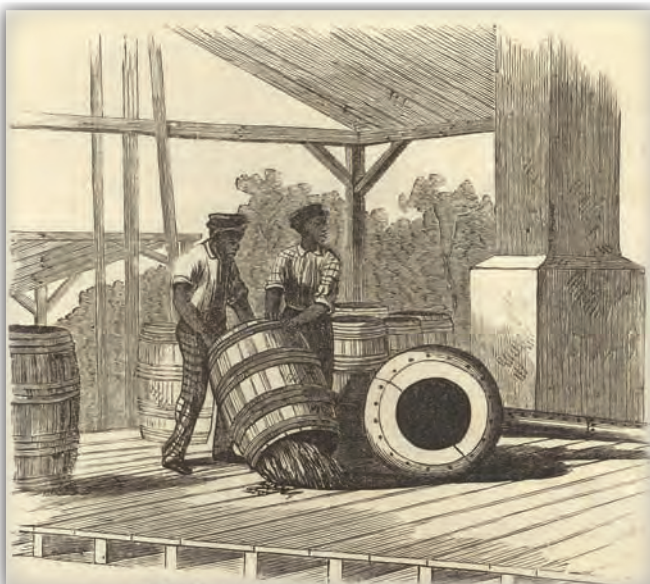
Charging the Turpentine Still (courtesy of Fort Bragg Department of Public Works).
