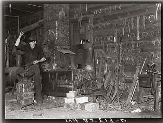
Arrangement of Blacksmith's Workspace. The anvil and forge are within a step of one another. Adjacent areas contain hand tools and raw materials. Vermont, 1937 (Library of Congress).
