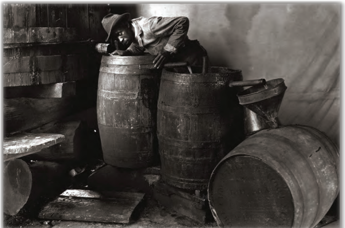
The Traditional Method of Gauging Distillation Progress: Listening to the Sound of the Heated Gum. The spirits are being double-separated. Unknown Location and Date (U.S. Forest Service).
