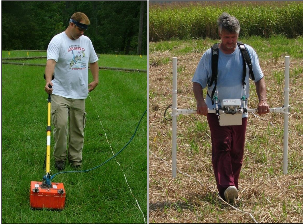
Figure 1. Use of a GSSI 400 MHz antenna detached from the SIR3000 cart (left) and use of a Bartington Grad601 dual gradiometer (right) (neither photo taken during this study).
