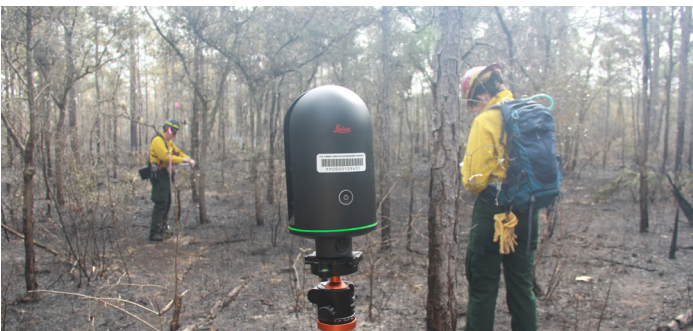
Fuel sampling and terrestrial lidar scanning of a research plot at Eglin AFB after a prescribed burn in March 2023. Credit: Mary Neil Armstrong, Southern Fire Exchange.
