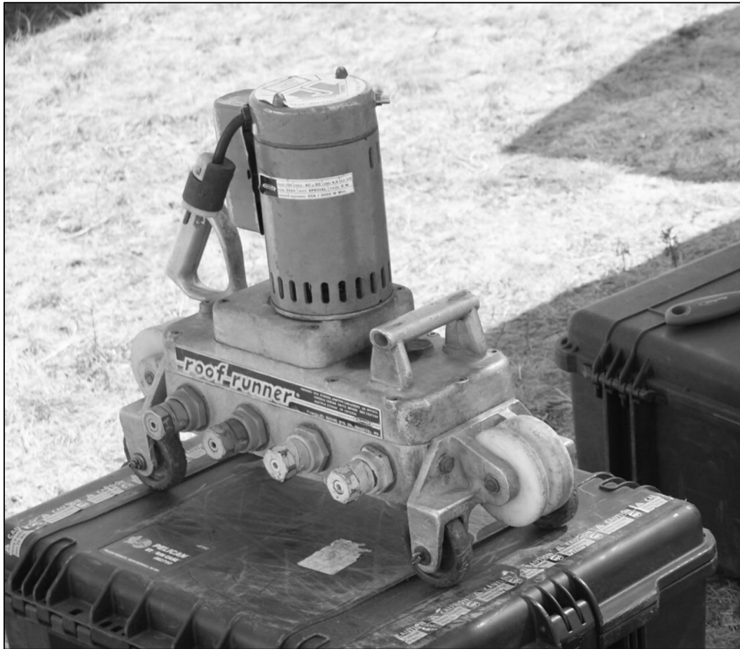
Figure 262. A “Roof Runner” machine used in the installation of the MR-24 roof, 2011 (Rider di, https://en.wikipedia.org/wiki/Roof_seamer#/media/File:Roof_runner.jpg ).
