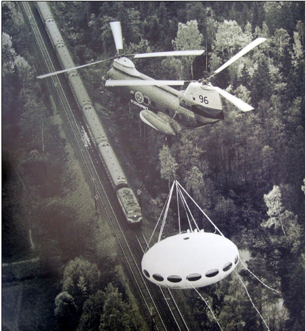
Figure 169. A Futuro house being transported by helicopter, Sweden, 1969 (Craig Barnes, "Futuro History," accessed Sept. 5, 2019, " http://www.futurohouse.co.uk/futuro-history.html ").
