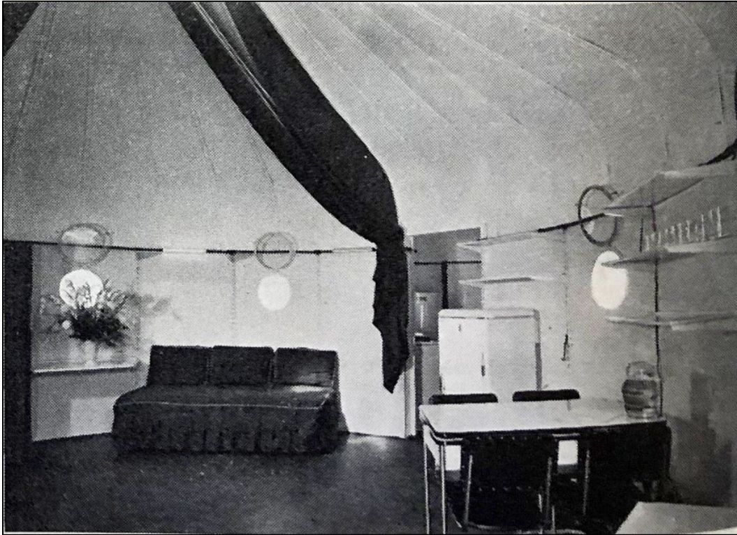
Figure 27. An interior view of a Dymaxion Deployable Unit showing the use of curtains as internal room dividers, 1944 (“Prefabricated Emergency Housing and Structures for the Armed Forces,” Prefabricated Homes 1-5 , (1944): 16–17).
