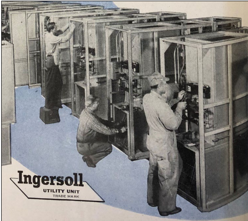
Figure 126. Three utility cores are being worked on at once in an Ingersoll factory, demonstrating the efficiency of production added by the core (Borg-Werner Corporation, "Ingersoll Utility Unit: Now in Volume Production! Prefabricated Homes 1-5 (1947): 2-3).
