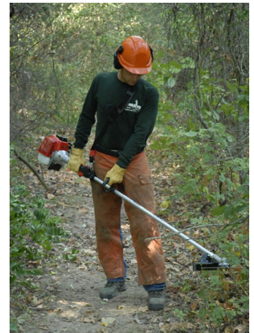
Many invasive species can be controlled using smaller handheld tools like this brush cutter with rotary blade allowing for easier transport for the mobile strike teams. Source: IPC
