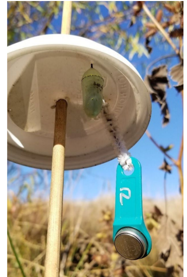
Monarch pupa attached to iButton temperature logger at Beale AFB, California. Photo by Stephanie McKnight, Xerces Society
