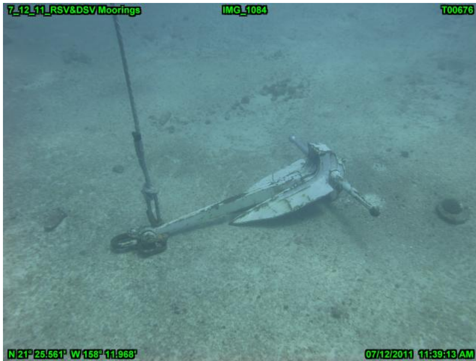
Figure 5. RSV anchor and mooring line.
