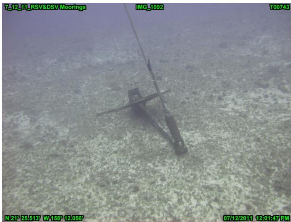
Figure 6. RSV anchor and mooring line.
