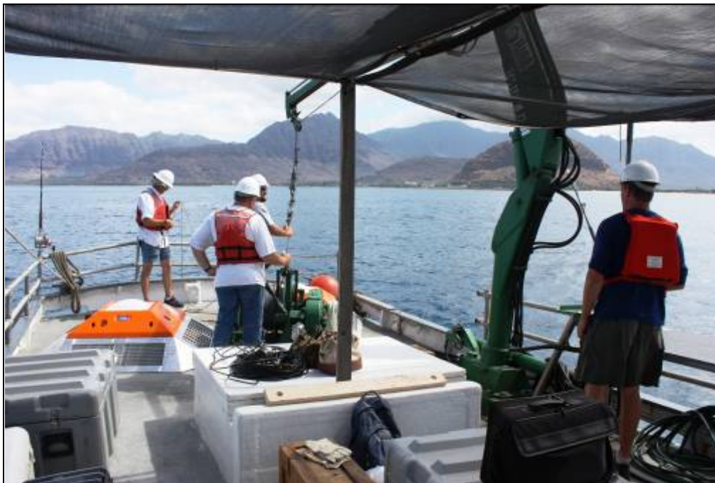
Figure 11. NDBC engineers aboard the University of Hawai'i Research Vessel KLAUS WYRTKI deploying a shallow-water ADCP mounted in a Trawl Resistant Bottom Mount at the Ordnance Reef (HI-06) site, July 25, 2009.
