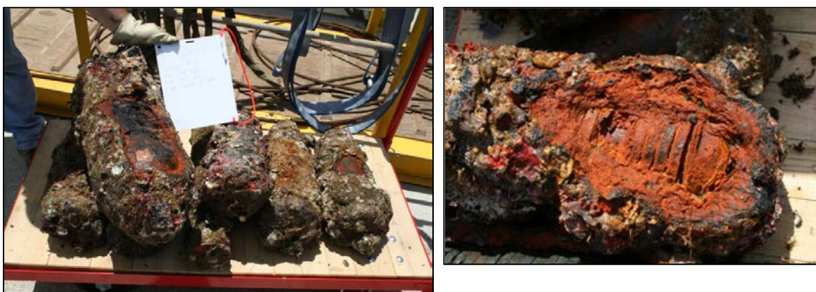
Figure 6. Photos showing varying degrees of encrustation on munitions recovered at Ordnance Reef (HI-06). The photo at right shows encrustation on a fragmentation bomb. Some of the encrustation on this bomb was removed during recovery operations, revealing the thickness of this encrustation.
