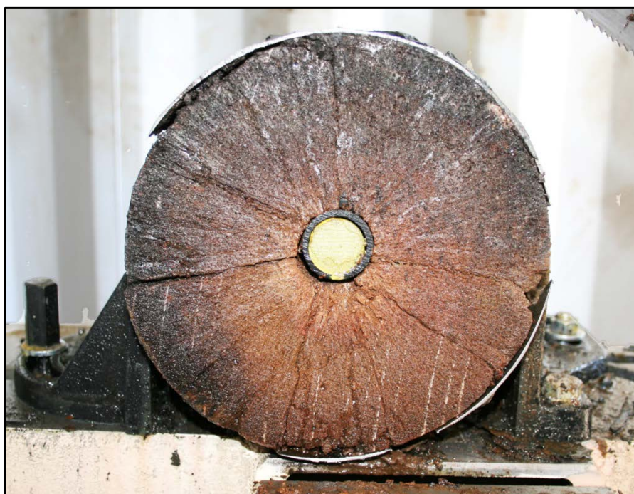
Figure 7. A 100-pound bomb recovered during the ROUMRS technology demonstration. This bomb was cut to expose the main explosive charge (large area with cracks) and booster (at center). Note that much of the metal bomb casing was completely corroded away (and is missing at lower left and center right), although the explosive appears relatively intact. Artillery projectiles, which have thicker shell walls, were largely intact, but many had leaked, allowing water to enter the explosive.
