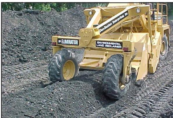
*An Eliminator mixes contaminated soil and microbe-containing soil to facilitate soil cleanup.*
