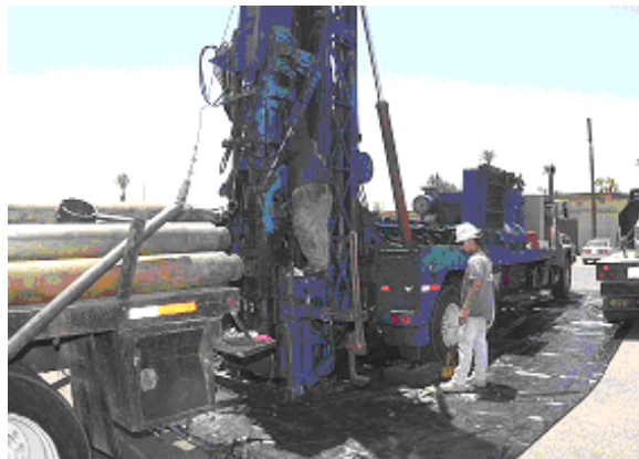
Taking soil samples from the Luke service station as part of an effort to prevent potential contamination.
