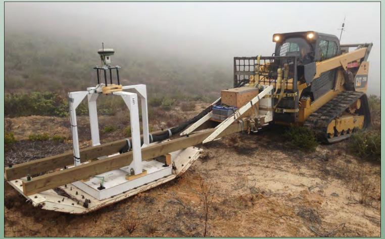
(Photo courtesy of USACE, Sacramento District) Advanced electromagnetic induction sensors are used to distinguish unexploded ordnance from scrap metal at a munitions response site at Fort Ord, California.
