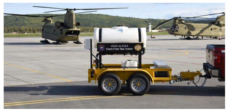
The foam-free test trailer will be used to ensure that fire trucks and pumpers designed to respond to aviation fuel fires are functioning at their peak, while being protective of the environment. (Photo by Brian Schlumbohm)
