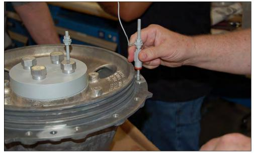
As part of the ESTCP Demonstration, a UH-60 output housing is masked, Tagnite anodized and sealed with Rockhard. (Photo courtesy of U.S. Army)
