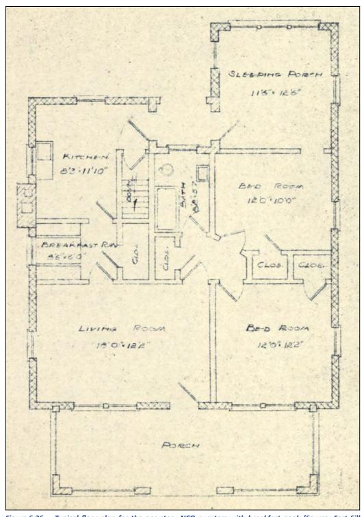
Figure 6.26. Typical floor plan for the one-story NCO quarters with breakfast nook (Source: Fort Sill Digital Archive 1800A\_B1822\_BB07\_B543).
