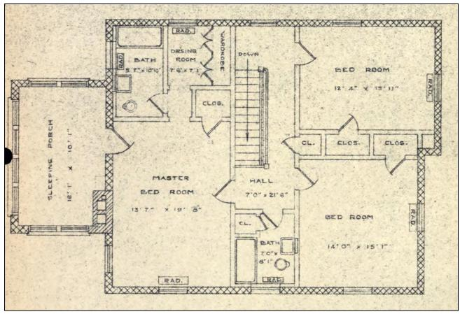
Figure 6.20. Typical second floor plan for company officer quarters (Source: Fort Sill Digital Archive 5000A\_B5083\_BB07\_B51\_PF158).
